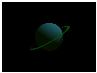
When you add a "filter" to a color, the color will let some light through. In this case, the color is green and the filter is .5, so any green light is let through at 50% of its normal strength. Take a look at the shadow that the ring is casting on the sphere. Where it was black, it now has a greenish tint to it.
